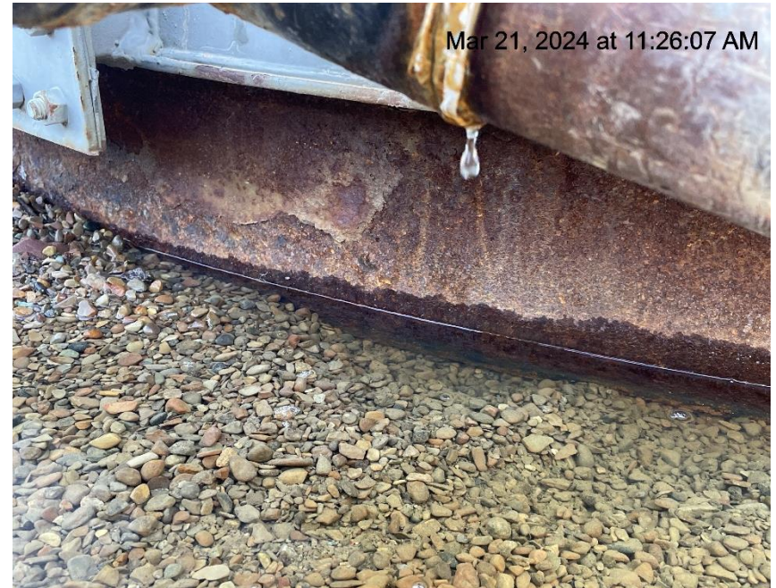
Photo # 865 Mechanical condition – fluid leaking from tank valve
