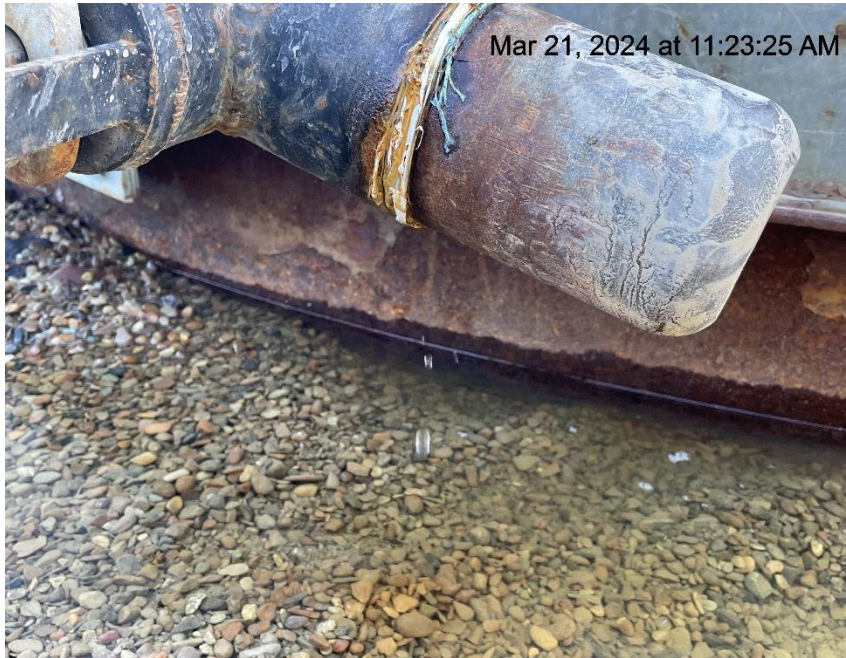
Photo # 864 Mechanical condition – fluid leaking from tank valve
