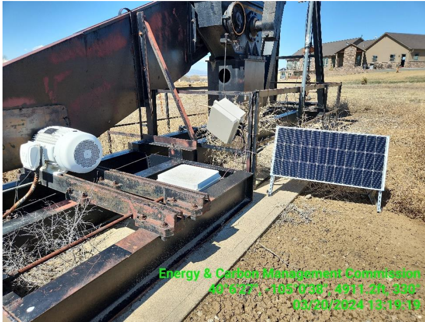
Photo 7 Prime mover(electric motor)/ monitoring equipment.
