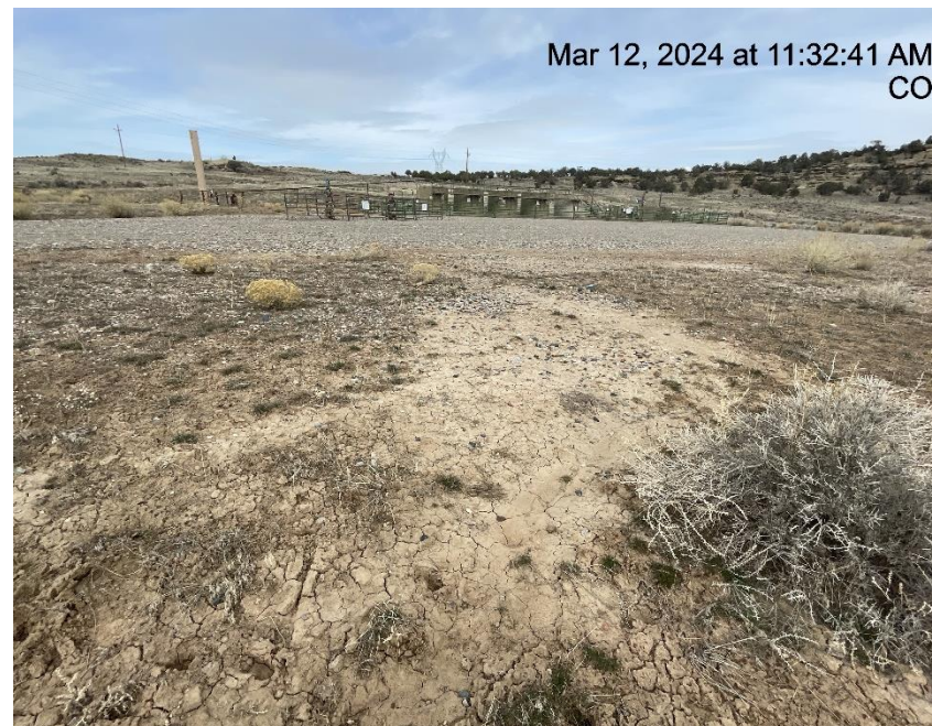
Photo # 9435 Failure to minimize erosion & transport of sediment off location/insufficient BMP's (E/SE area of location)
