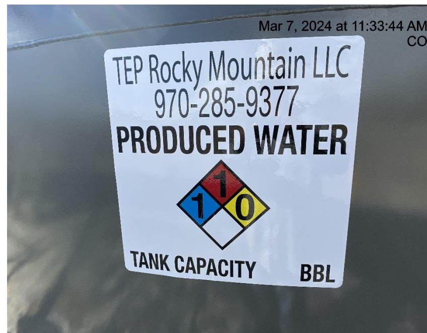
Photo # 9055 Tank label lacks required information
