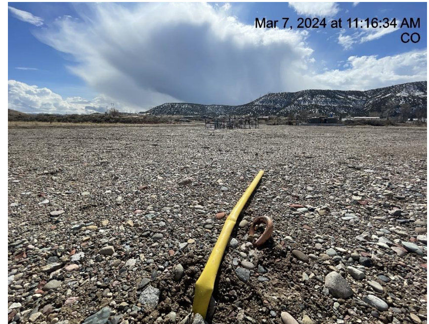
Photo # 9057 Improperly marked deadman
