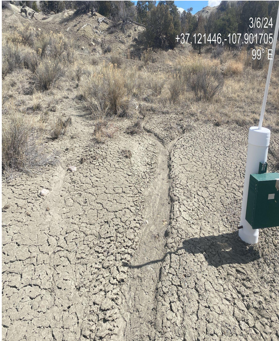
Photo 4. View of rill erosion forming in the southeast and northeast portions of the disturbance.
