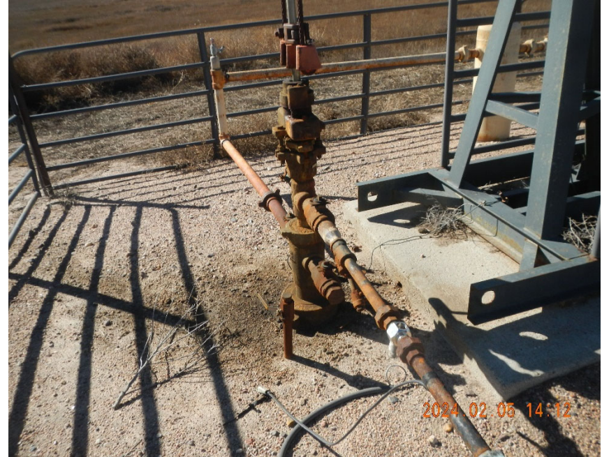
4. Stained soil at wellhead 02/05/2024.
