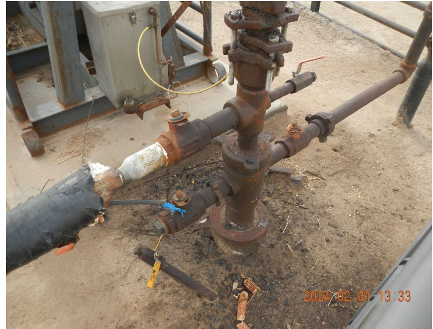
2. View of wellhead. Note stained soil around wellhead.
