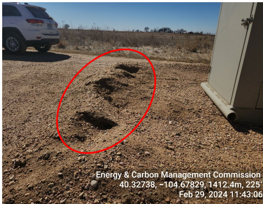
Photo 5: Damaged berm
