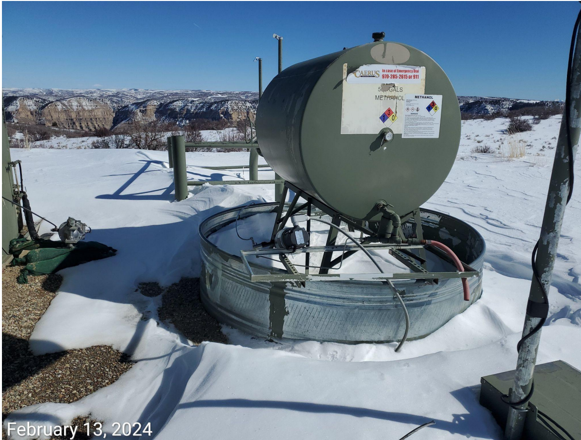
Photo 3: Wildlife protection BMPs missing or insufficient at the methanol tank containment BMP.
