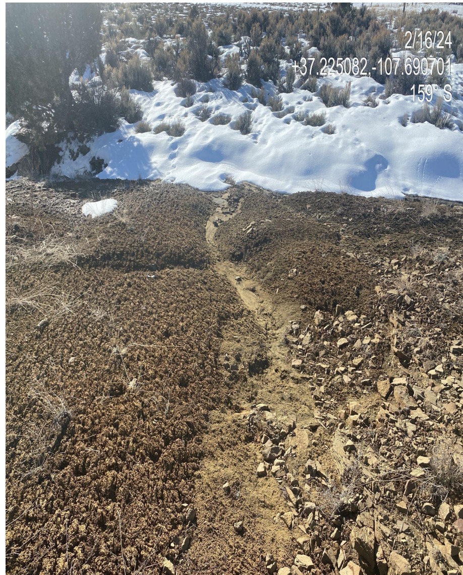
Photo 3. View of rill erosion forming in the southern interim reclamation area.
