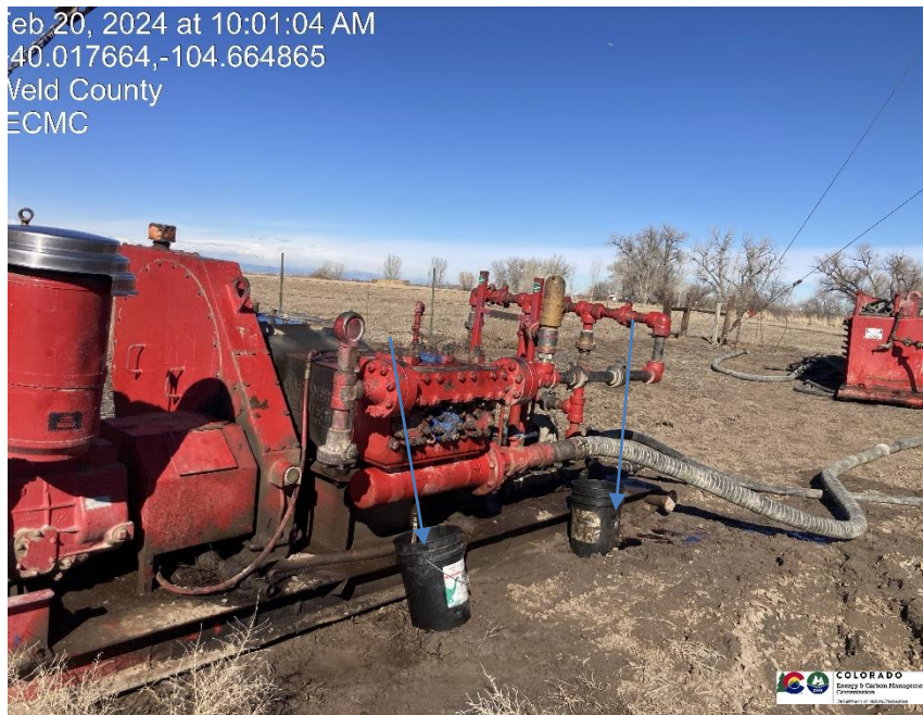
Pic 1 oil was observed on ground, no stormwater containment
