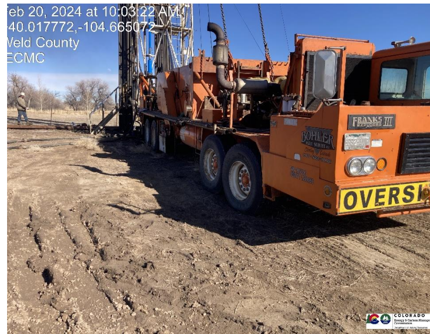
Pic 6 No stormwater containment under rig
