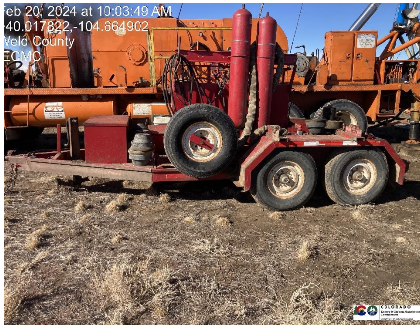
Pic 7 No stormwater containment under accumulator
