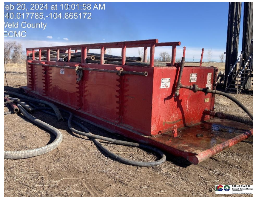
Pic 4 Rig tank is not grounded.
