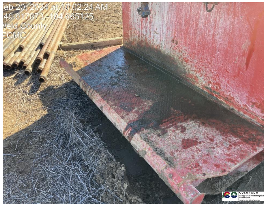
Pic 5 No stormwater containment on rig tank
