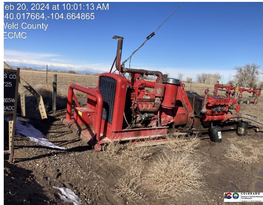
Pic 2 Rig pump is not grounded.
