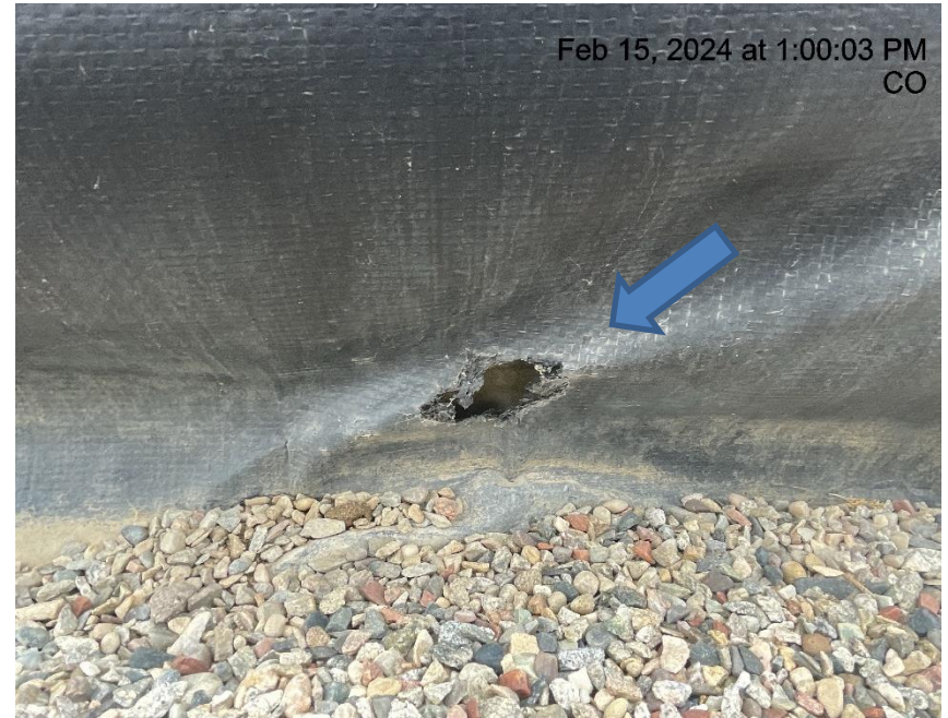
Photo # 6851 Hole in liner/liner needs maintenance
