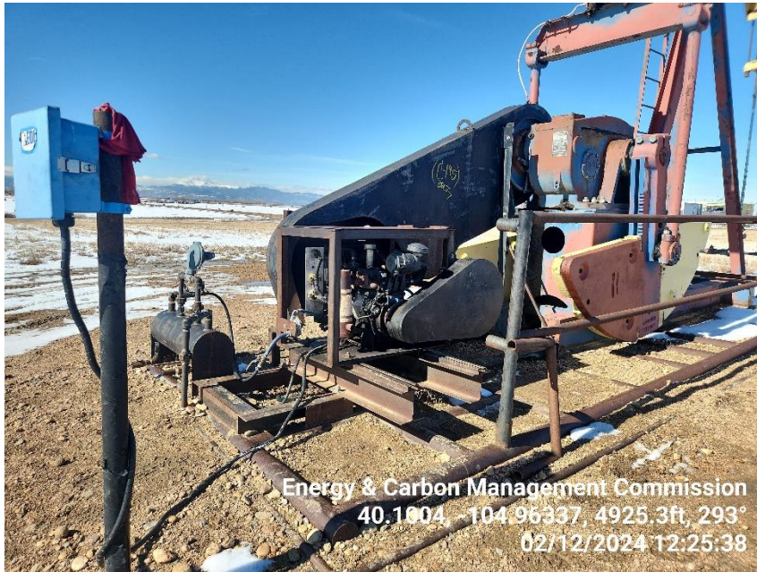
Photo 5 Prime Mover/Gas Engine.
