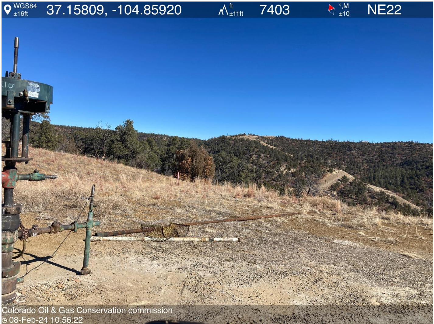
PHOTO 5: UNUSED EQUIPMENT LEFT ON LOCATION (PUMP AND TBG). COMPLY WITH RULE 606, REMOVE UNUSED EQUIPMENT. CA DATE 3-8-2024.
