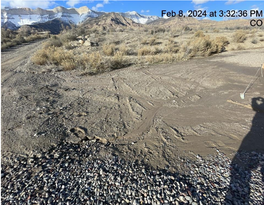
Photo # 5611 Erosion & transport of sediment onto location/insufficient BMP's/insufficient run on/runoff controls
