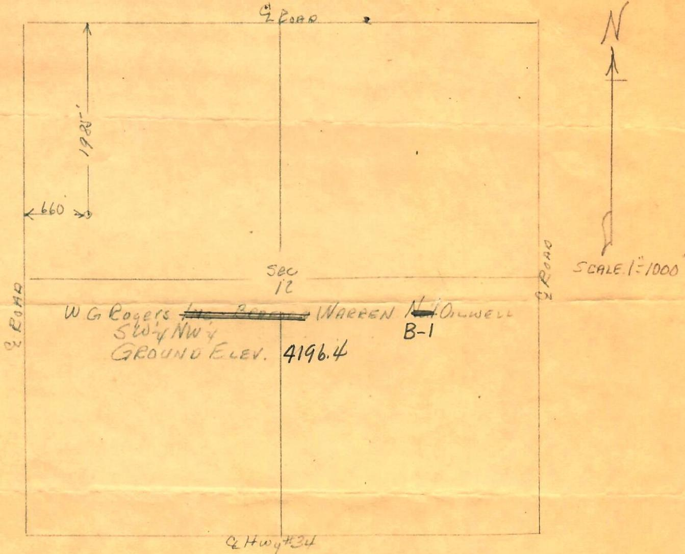
I hereby certify that the above plat is an accurate representation of a correct survey showing the location of W.G. Rogers ~~Inc.~~ ~~Warren N Oilwell~~ Oilwell in SW 1/4 NW 1/4 Sec. 12 T2N R49W 6PM. The elevation of the ground at the stake is 4196.4 feet above sea level from U.S.C.&G. Bench Mark.
