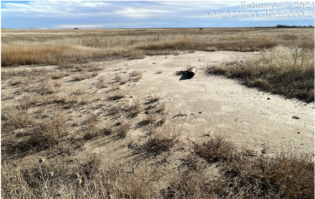
Photo 2. Facing east toward the location. This area approximately 50'x50' has no vegetation and soils appear impacted from historic release at the wellhead.
