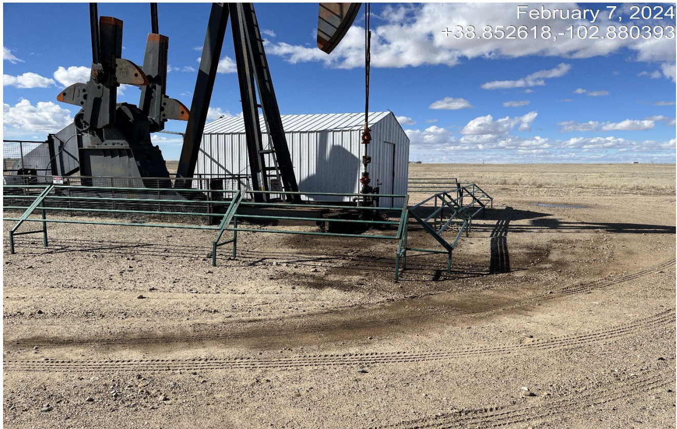
Photo 2. There is oil stained soils around the wellhead that must be cleaned up..
