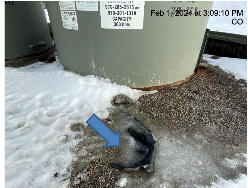
Photo # 5410 Possible tear in base of secondary containment liner
