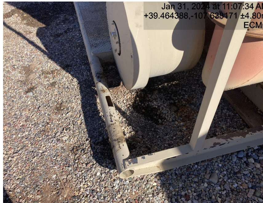
Staining behind separator
