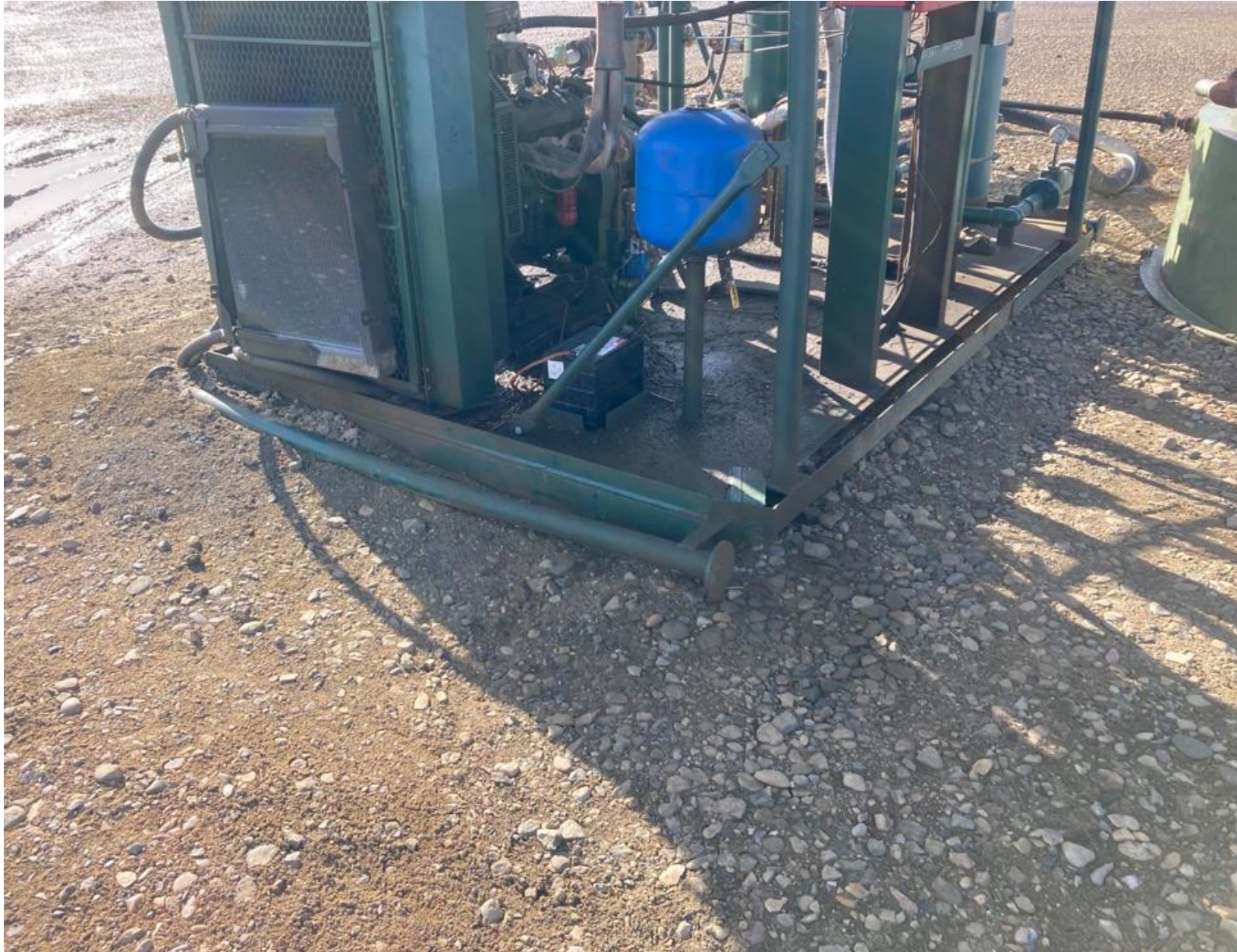
PHOTO 2: THE SOIL STAINS HAVE BEEN REMOVED AND THE ENGINE SKID CLEANED. THE PANEL DOOR HAS BEEN REPLACED ON THE HOUSING AND THE UNUSED PIPING ON THE GROUND REMOVED.
