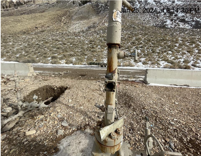
Photo # 4109 Open valve leaking gas on the MF04B-3 wellhead
