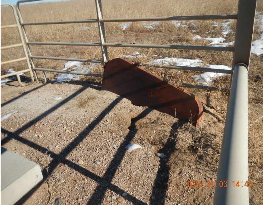
3. Belt guard removed and on ground inside fencing.
