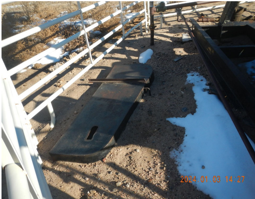
3. Belt guard on ground inside fencing.
