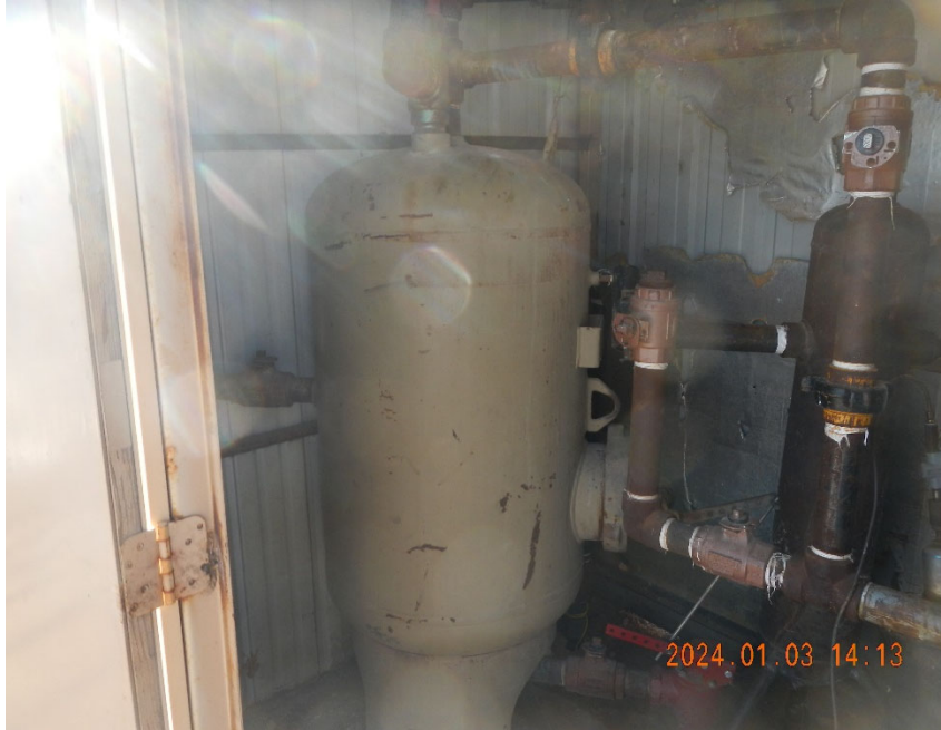
5. Vertical separator inside remote shed.
