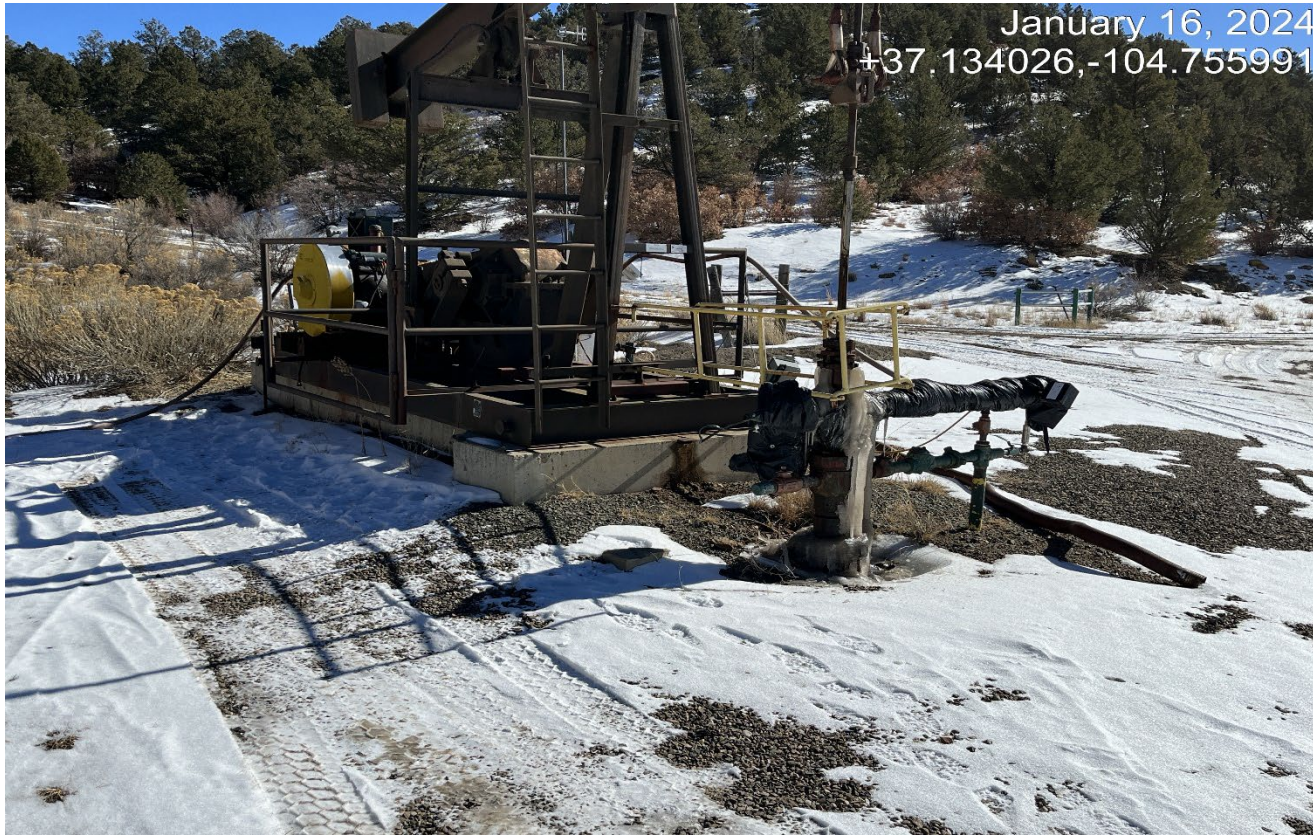
Photo 3. There is ice build up from a dripping leak at the wellhead.
