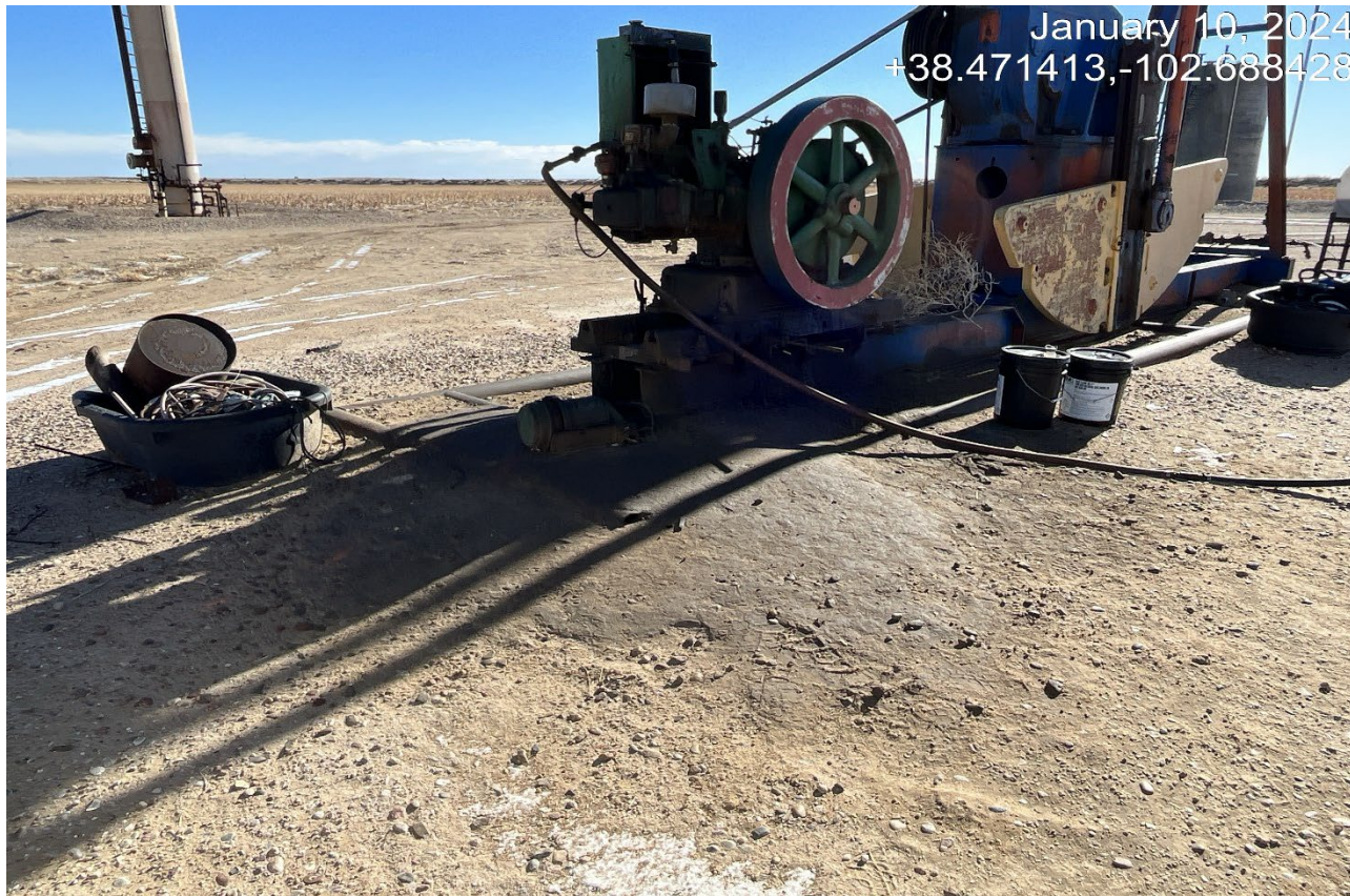
Photo 4. There is oil stained soil next to the engine pumpjack that needs to be cleaned up.
