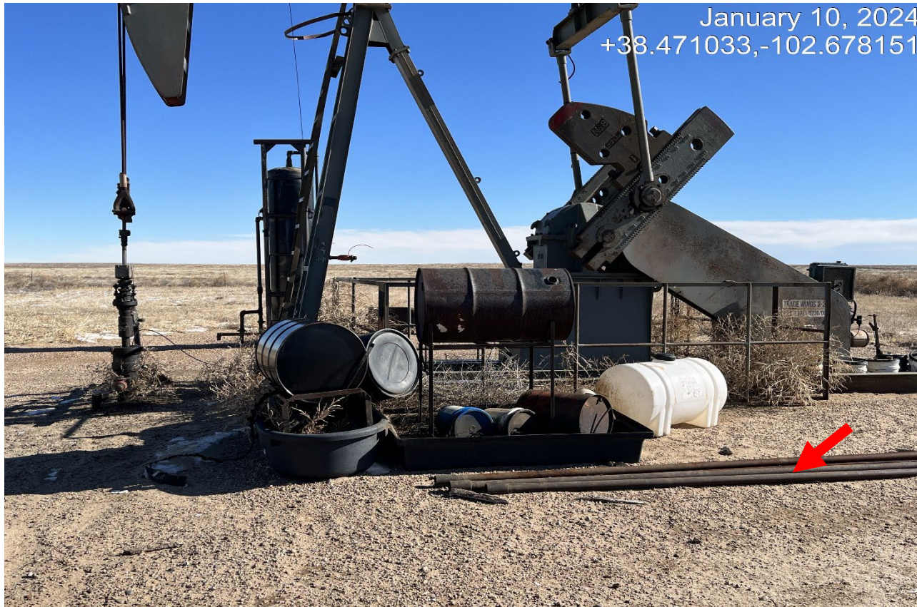
Photo 8. Facing toward the pumpjack. Unused pipe and containers need to be removed.
