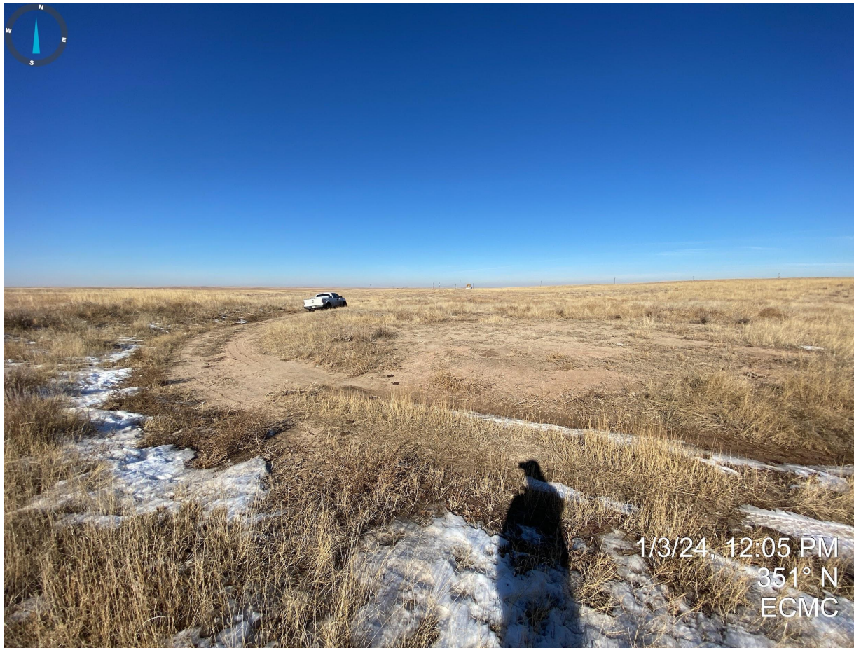
Photo 2. Taken south of the location, facing north. Photo illustrates that the access road and former location have not been regraded or contoured to reflect pre-disturbance conditions.
