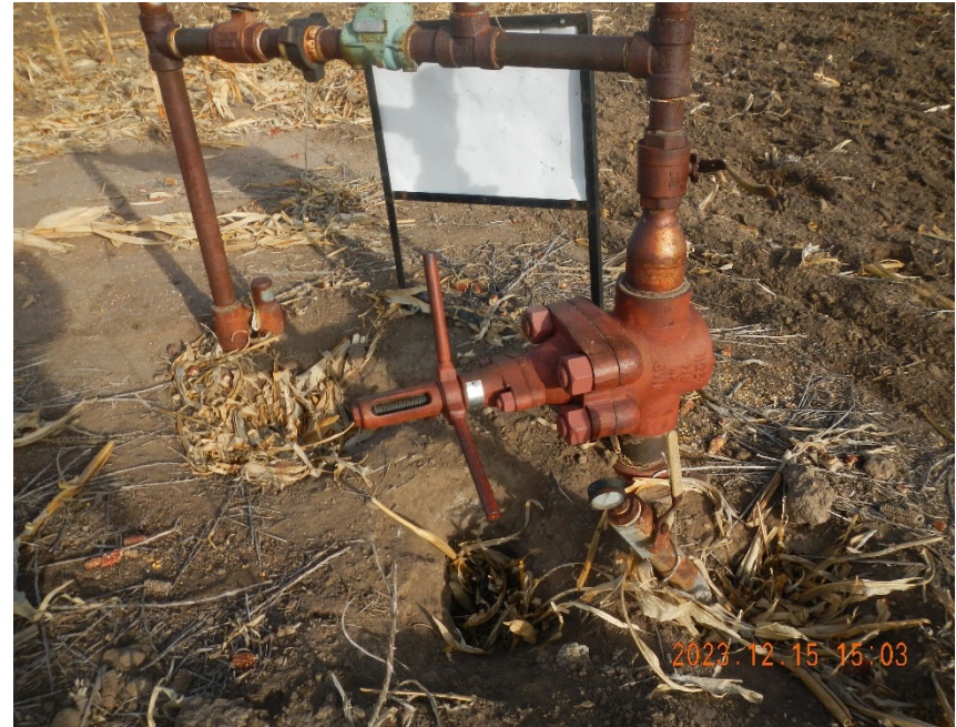
2. View of wellhead. Note capped flowline riser.
