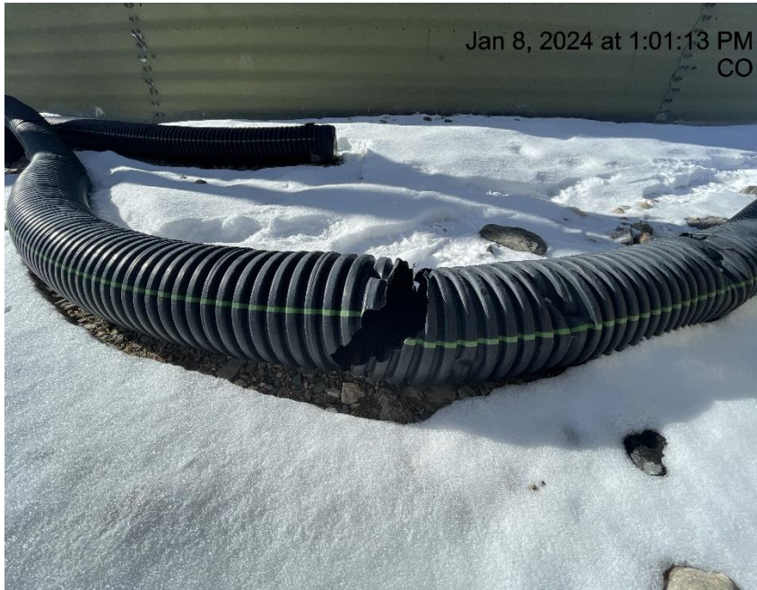
Photo # 2038 Hole in flowline heating insulation/wildlife hazard
