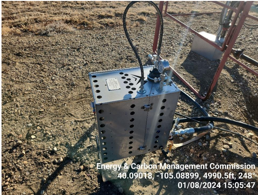
Photo 3 Fugitive gas recovery device.
