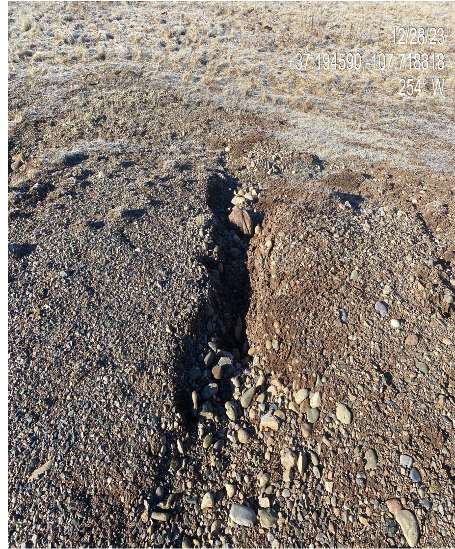
Photo 2. View of rill/gully erosion forming on the western edge of the disturbance. Current round river rock stormwater BMPs are not adequate.
