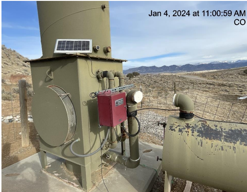
Photo # 1727 Unused equipment – ECD disconnected
