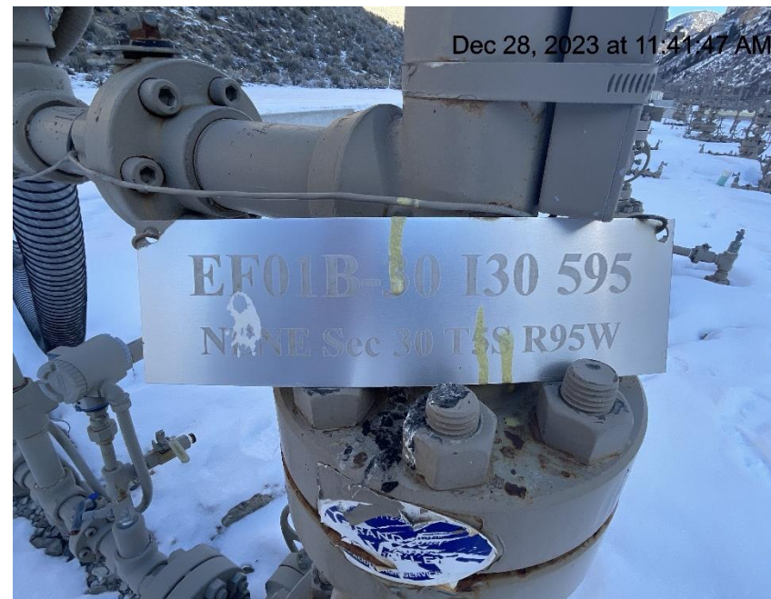
Photo # 1117 Wellhead signs lack required information
