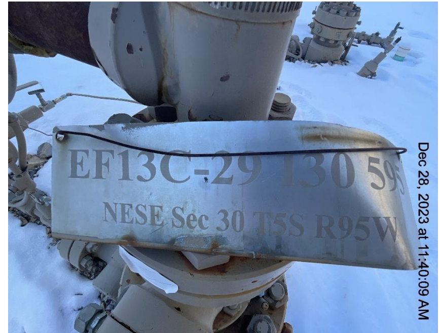
Photo # 1115 Wellhead signs lack required information
