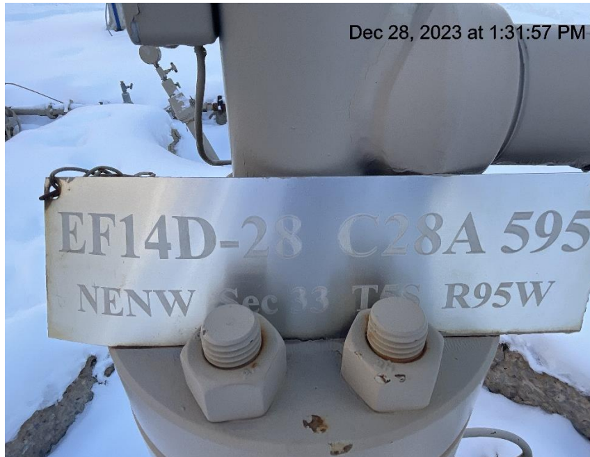
Photo # 1291 Wellhead signs lack required information
