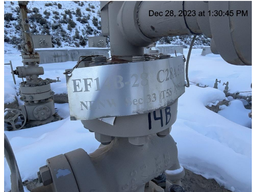
Photo # 1290 Wellhead signs lack required information
