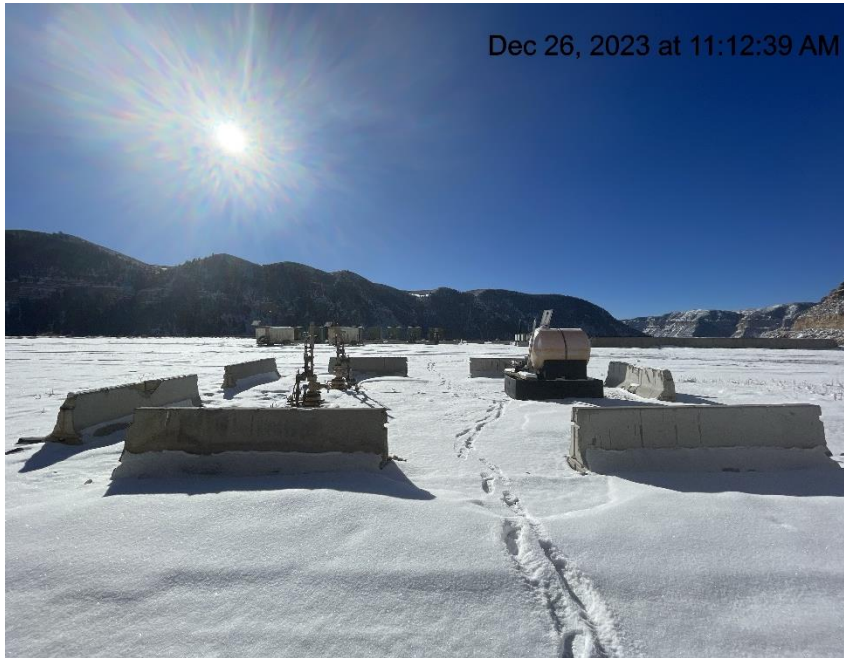
Photo # 761 Wellheads lack required signage
