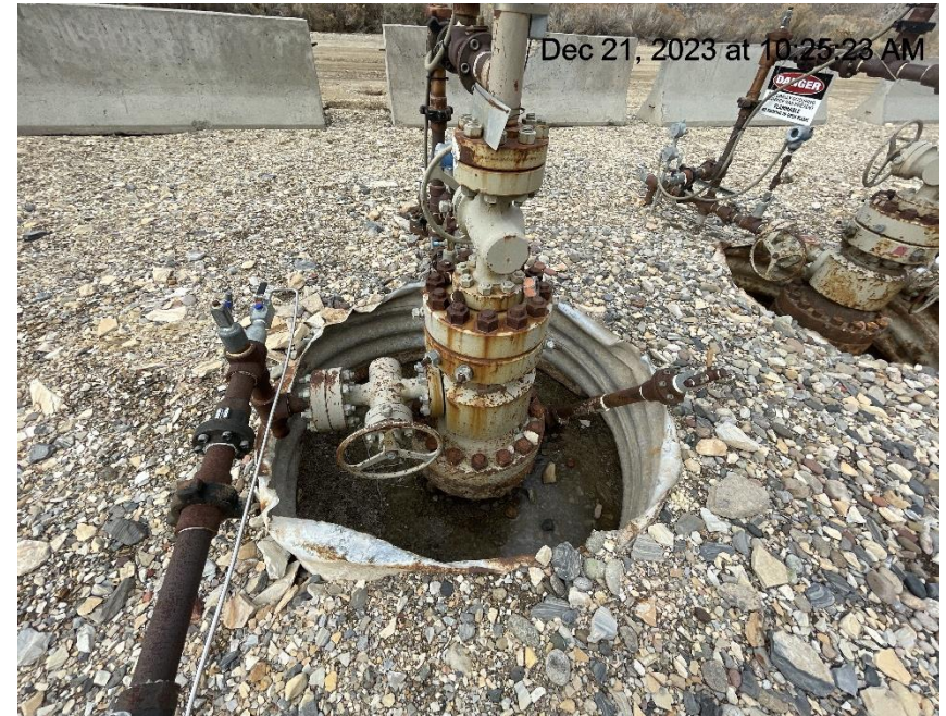
Photo # 427 Open wellhead cellar
