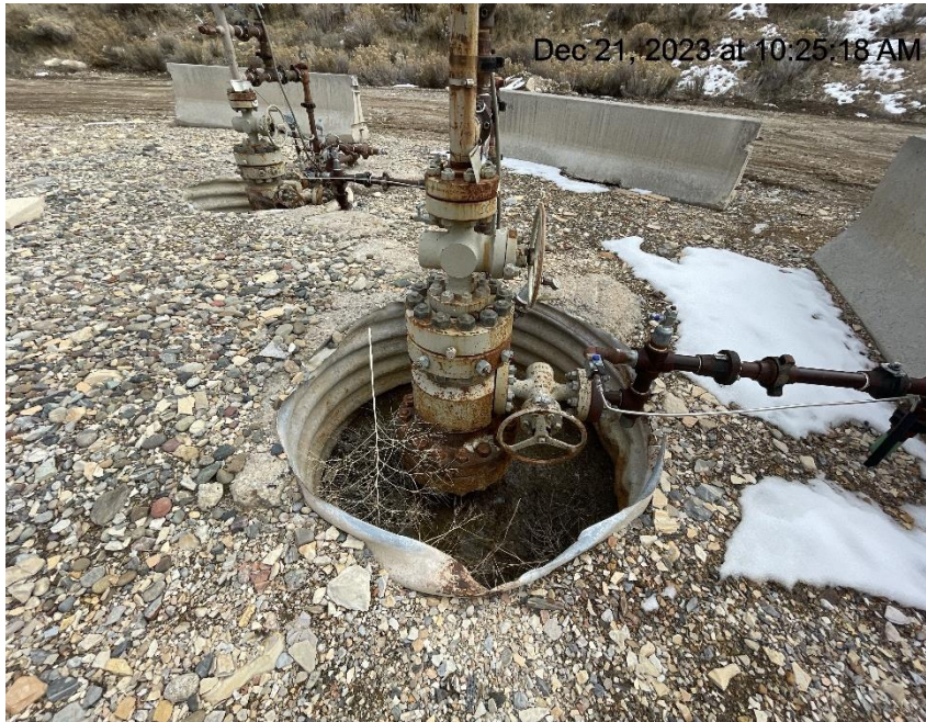
Photo # 426 Open wellhead cellar
