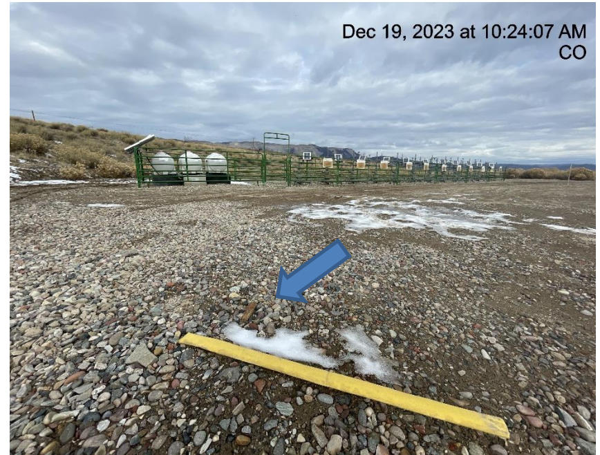
Photo # 105 Unmarked/improperly marked deadman
