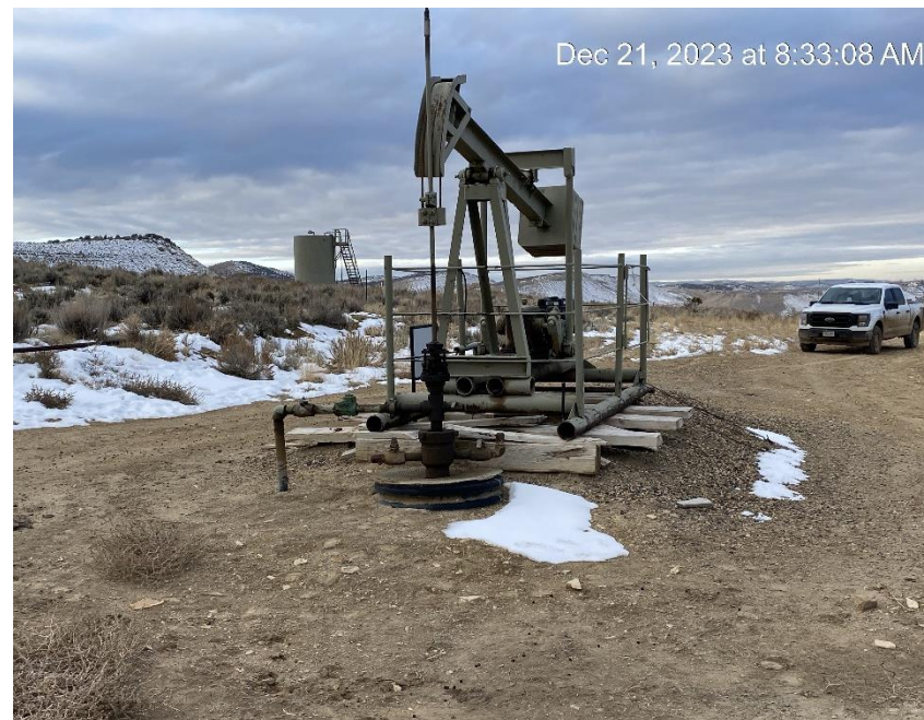
Pumping unit with production tank
