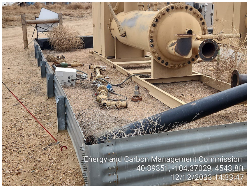
Photo 15 – Separator is open to Atmosphere. Unused Meter Tube, Pipe, Fittings and Heat Stack. Unmarked Risers
