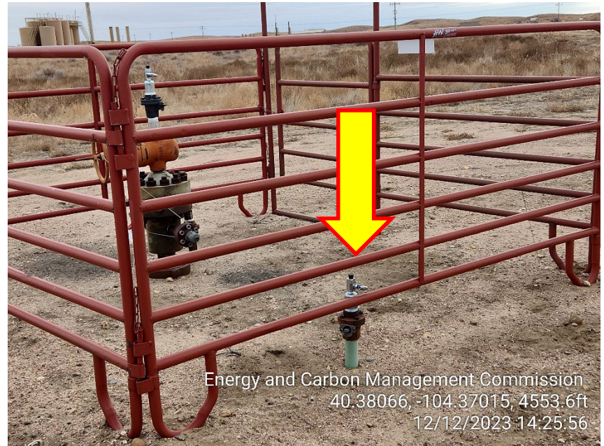
Photo 10 – Unmarked Riser at Wellhead
