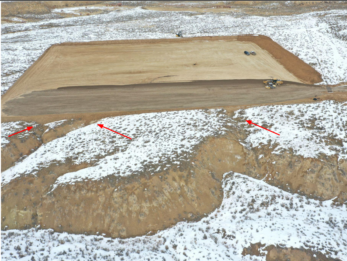
Photo 12: Photos 12-14 taken with use of a sUAS. Photos show Rimrock Gulch, and drainages where fill material has been placed within (arrows). Refer to Photos 9 & 10 for additional comments.
