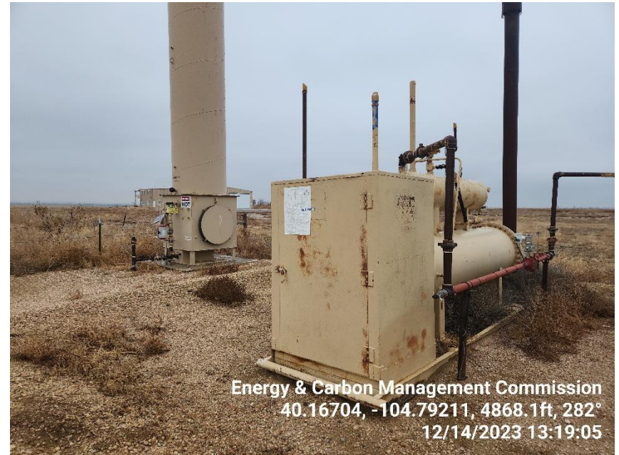
Photo 14 ECD & Horizontal Heated Separator.
