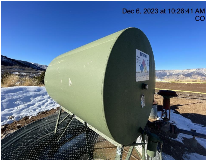
Photo # 8613 Methanol tank improperly labeled/lacks required information
