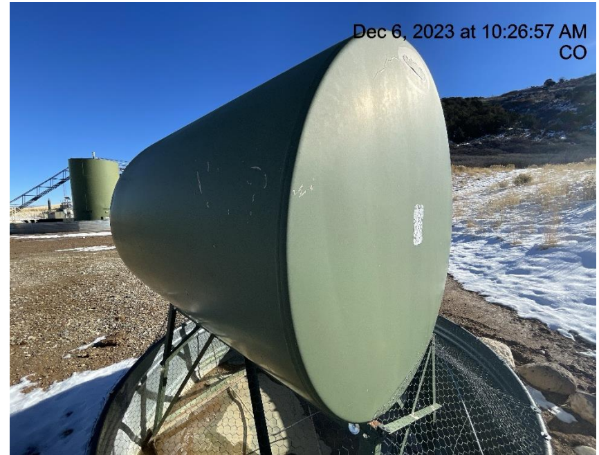
Photo # 8614 Methanol tank improperly labeled/lacks required information
