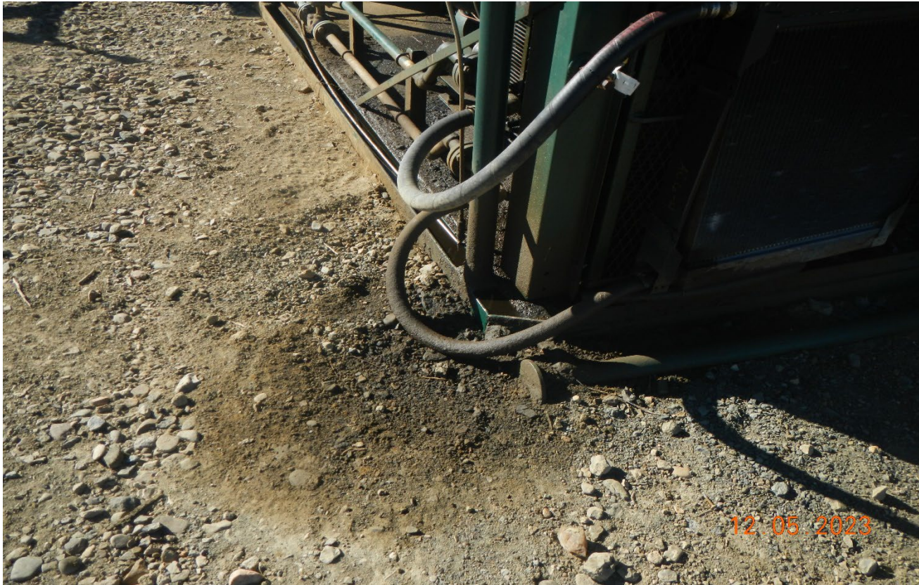
Photo 4. The engine skid is full of oil and has spilled onto the ground..
