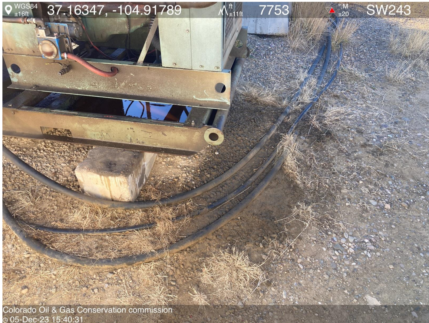
PHOTO 5: AREA OF IMPACTED SOIL NEAR PRIME MOVER SKID. Conduct maintenance on equipment, cleanup stained material and review self inspection processes. COMPLY WITH RULE 1002,.(2).D. CA DATE 1-5-2024.
