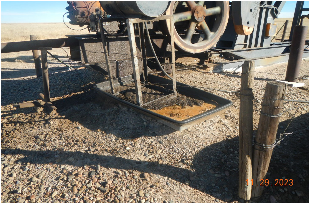
Photo 7. There is oily fluid in the containment next to the pump jack. Oily fluid has spilled onto the ground and needs to be cleaned up. Previous corrective action was not completed.
