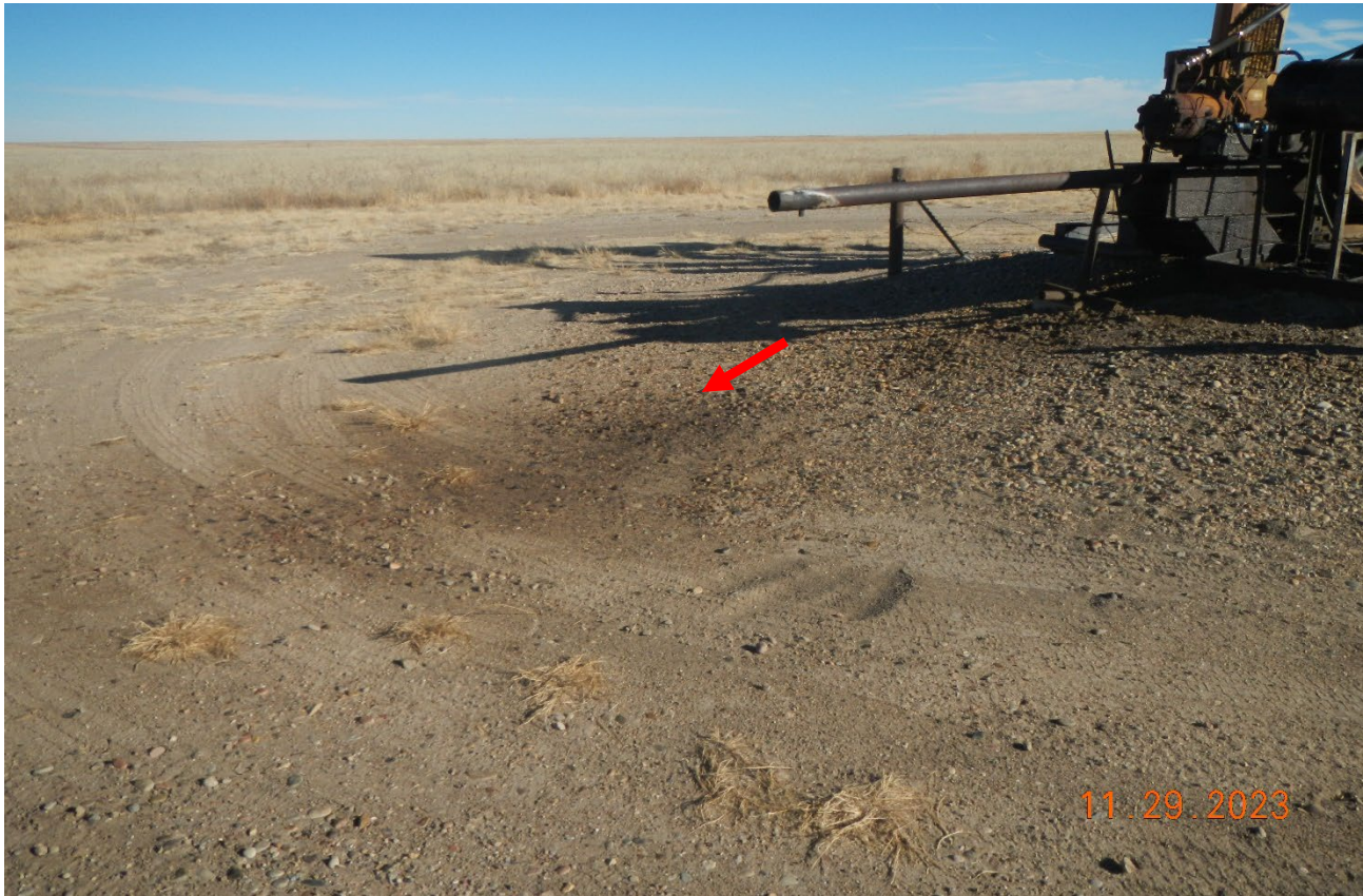
Photo 6. There is stained soils where exhaust is being blown on to the ground.
