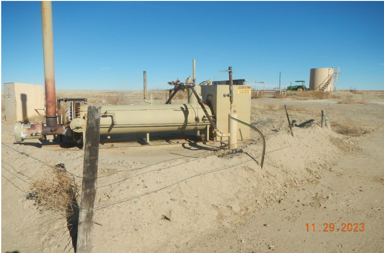
Photo 6. The northwest at the wellsite and production equipment. The fence around the equipment is inadequate to prevent livestock entry. Cattle track have previously been observed inside the 2 strand fence.
