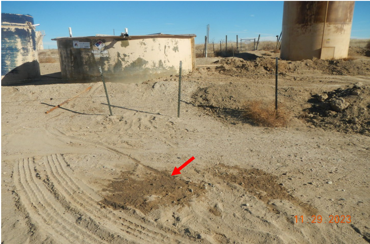
Photo 8. Facing toward the tanks at southeast side of the location. There is wet soils where the truck load out occurred and signs that the hose leak out water while disconnecting.
