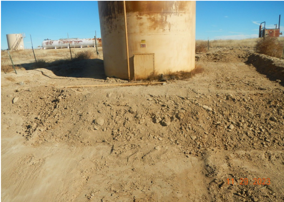
Photo 10. The berm pushed up is inadequate for secondary containment due to loose soils and inadequate size.
