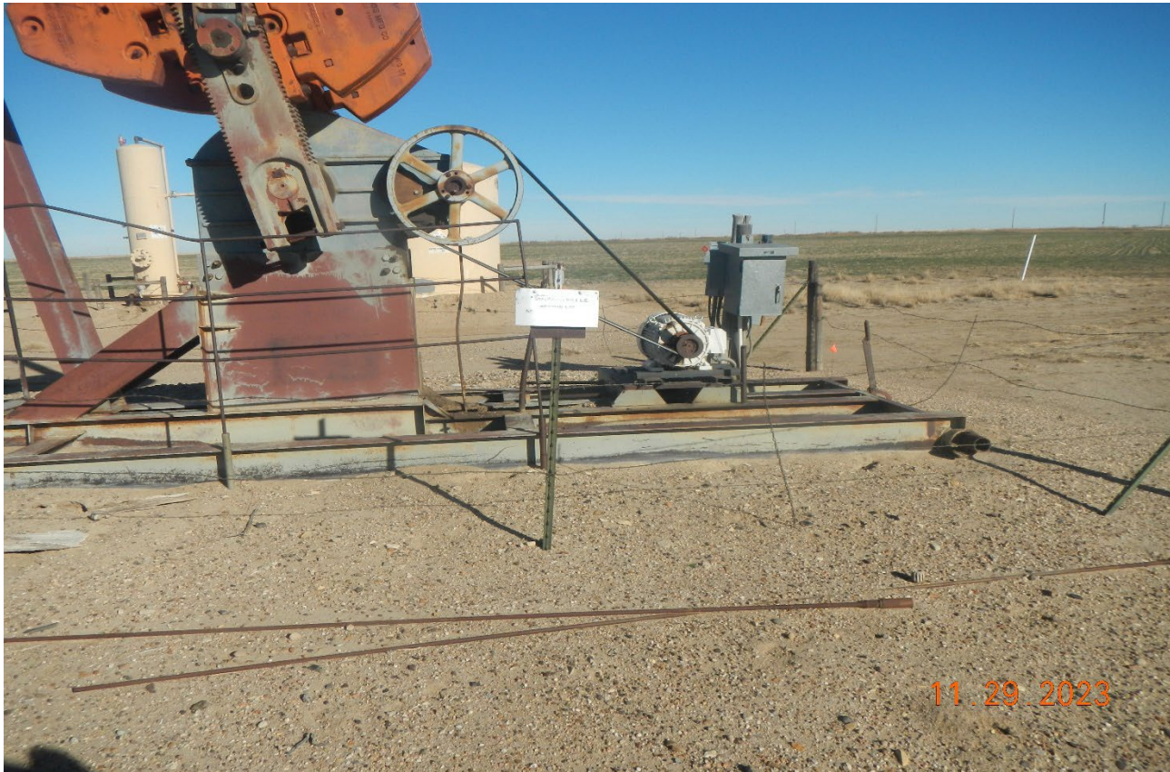
Photo 7. The well sign is faded and does not meet the signage requirements. Previous corrective action was not completed.
